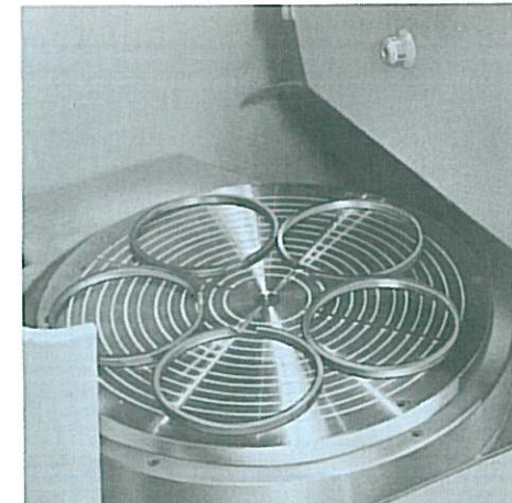
Split rings are quickly ground in lots of five
