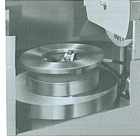
Here a fixture replaces the magnetic chuck
