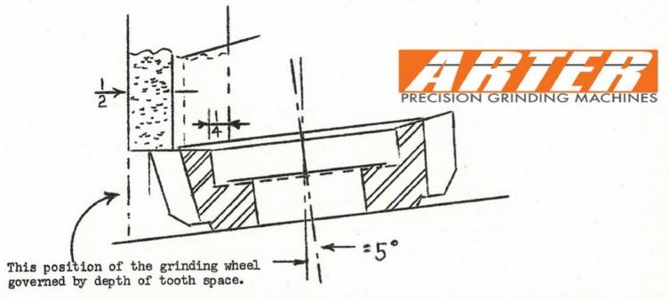
Disk and hub cutters can be sharpened on a rotary surface grinder, the cutter being centralized on and held by a magnetic chuck. Shank cutters should be held in a tapered-hole adapter centralized on the chuck.
